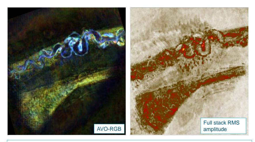
AVO-RGB blend on the left, on the right an RMS amplitude extraction from a 40mtr window centered on the horizon from the full stack. Bright blue colours are caused by higher amplitudes on the far stack indicating a potential shallow gas hazard in the meandering channel, though not in the funnel shaped amplitude anomaly.
