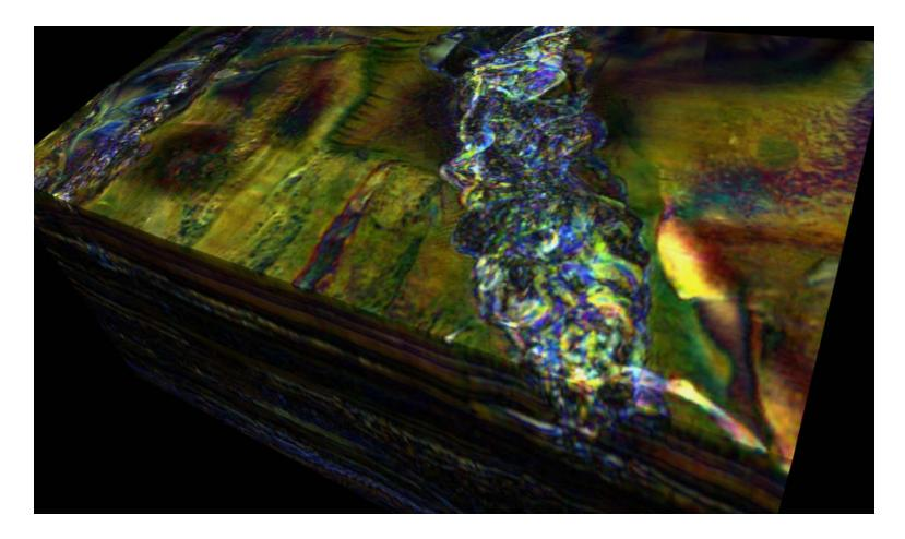
Shallow canyon fill with meandering channels showing blue colours indicating strong AVO response and likely shallow gas hazards.
