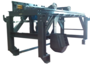
Sampler at the discharge of a conveyor belt
